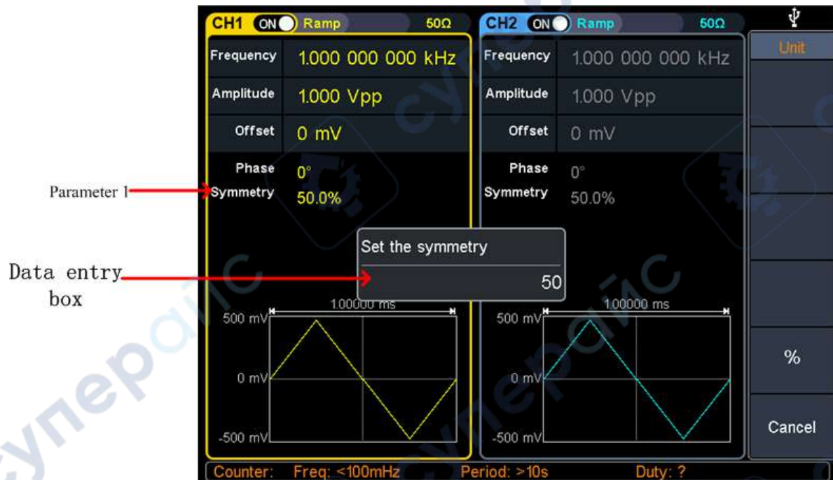
Figure 5-5: Set the symmetry of ramp wave
