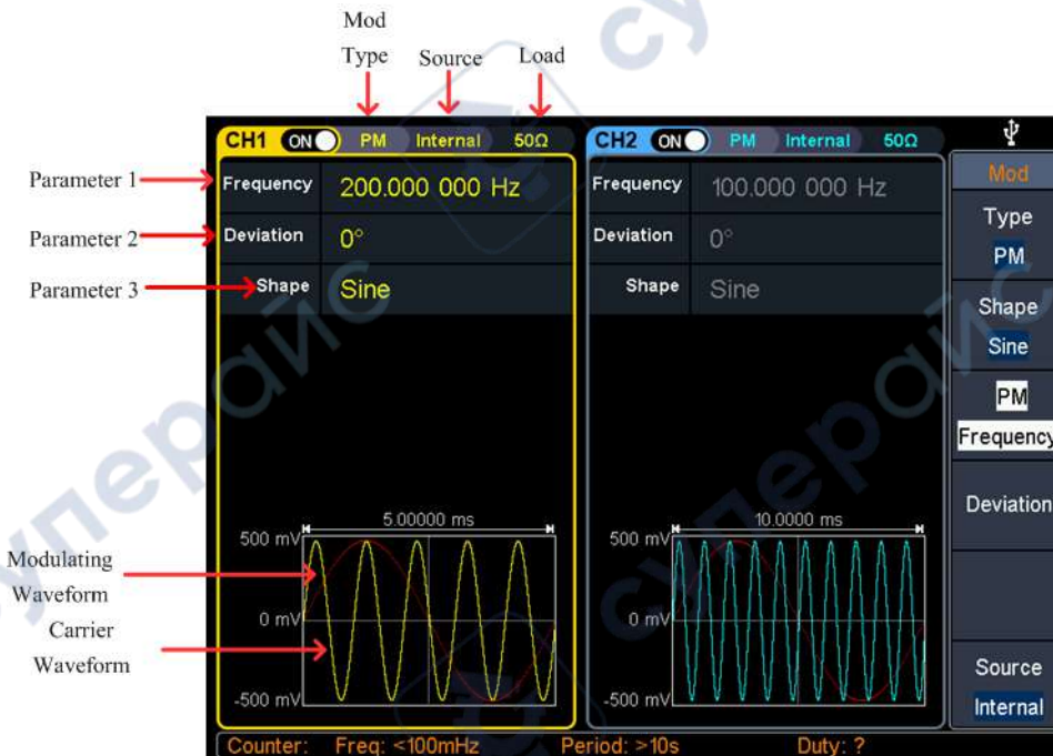
Figure 5-13: Phase modulation user interface
