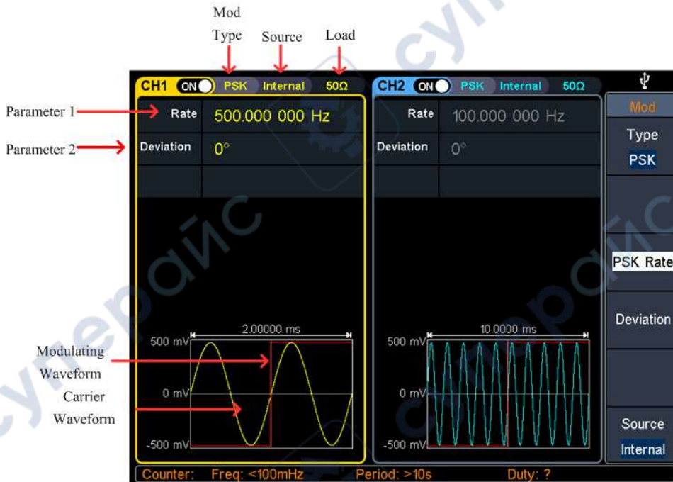
Figure 5-16 Phase shift keying user interface
